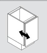
Rotate the rear spiral tech cam screw to adjust the door position (+ 3/- 2 mm).
