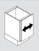
Rotate the front screw to increase or decrease the door overlay (+/- 2 mm).
