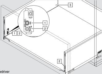
NOTE: Height, side and tilt adjustments must be achieved with a T20 Torx screwdriver
